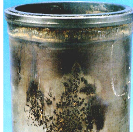
Item 1: Eroded by cavitation zone
