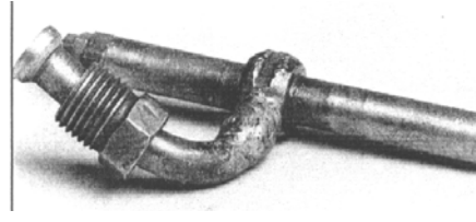
Repaired injector arms or body parts are unacceptable.
