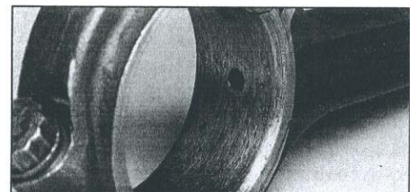
Damaged bearing surface
