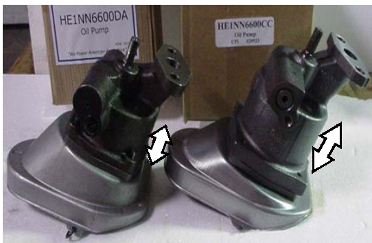
HE1NN6600DA HE1NN6600CC For 158-268 engines (notice the height difference!)
